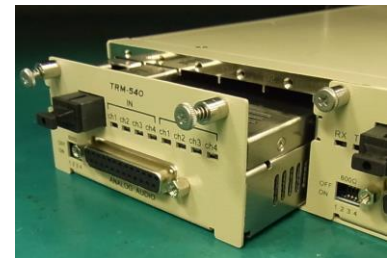
Figure.1 Optical converter installation
